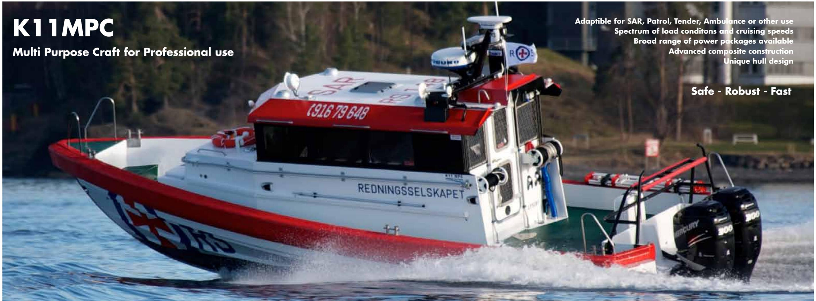
K11MPC is a light to medium displacement boat suitable for commercial use. K11MPC has a unique Kullmann type double curvature deep V hull similar to the award winning ones developed for fast heavy duty offshore rescue boats. The advanced modern hullshape coupled with the right power package will
